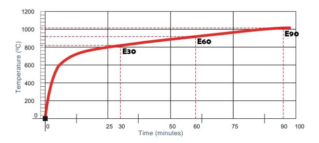
As minutes passed the trays began to deform because of the high temperatures, but they continued to be able to support cables sending an electrical signal. Depending on how many minutes the electrical system can maintain this electrical signal will determine how the system is classified: E30, E60, and E90.
