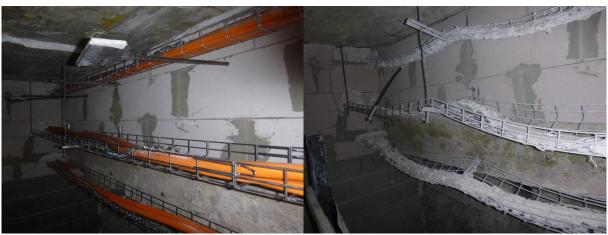
As the photos show, the structure of the EASYCONNECT trays that were tested, as well as the supports, did not collapse and they did not fully or partially come apart in any instance.
